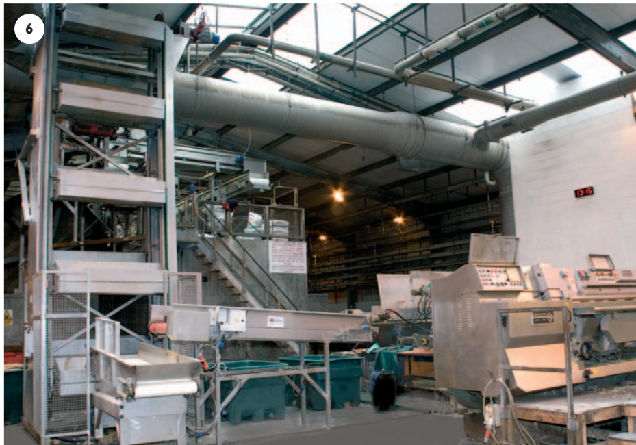
Figure 3: Operator clipping hides onto monorail chain conveyor feeding flesher
