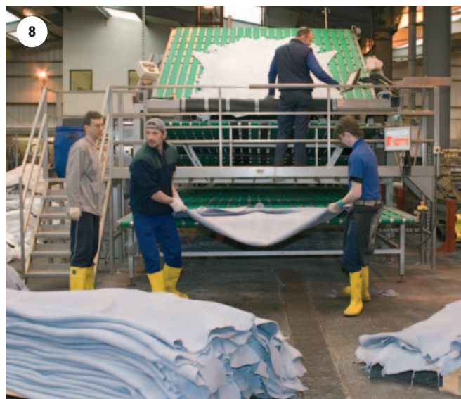
Figure 8: Operators stack folded hides from Feltre Viewer unit onto pallets
