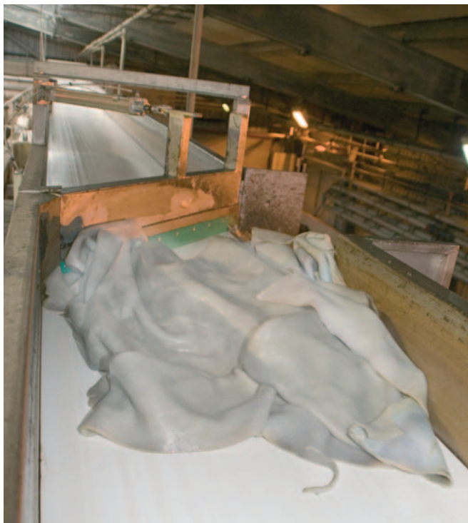
Figure 2: Hides are diverted off transport conveyor to drop into drum
