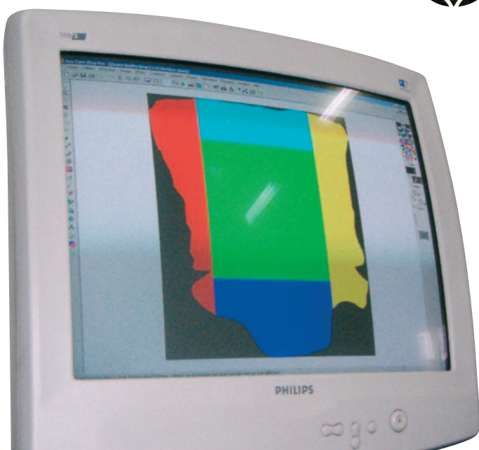
Figure 8: Parameters for different hide areas are set at the computer
