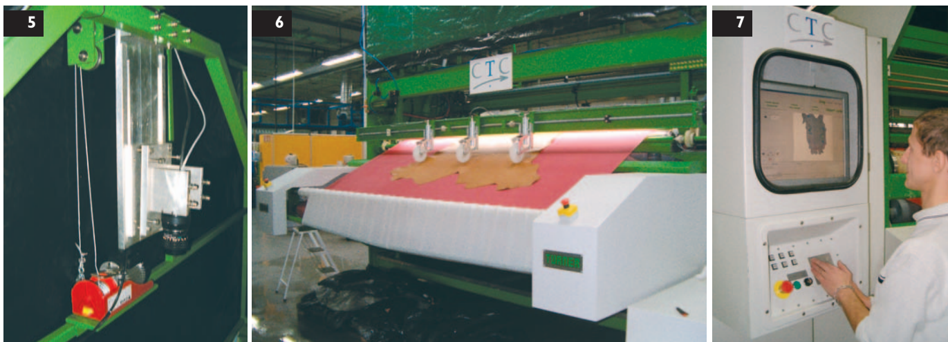
Figure 5: Digital camera on motorised mounting Figure 6: Hide passing out under thickness sensors Figure 7: Operator using trackerball at control console
