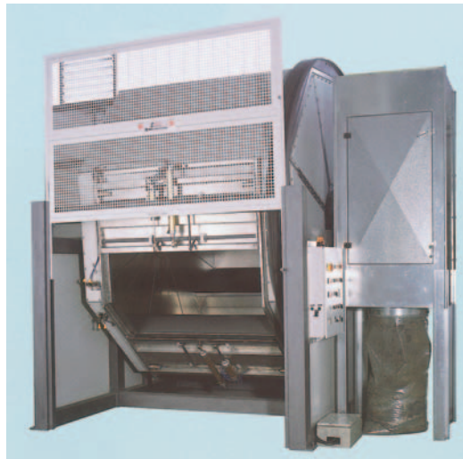
Octagonal milling drum with vertical safety sliding doors (Baggio)
