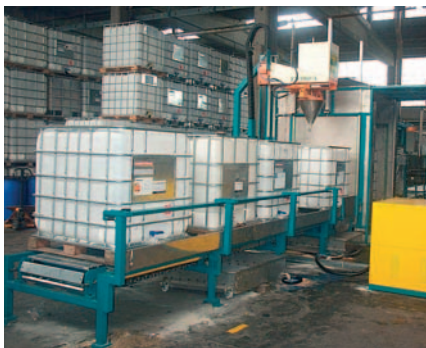
Multi-station automated line for washing, rinsing, draining and testing IBCs (C.E.B. Impianti)
