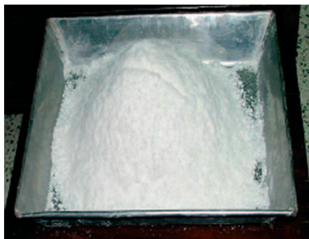
Panel 2: Formic acid neutralised Wasserglass powder
