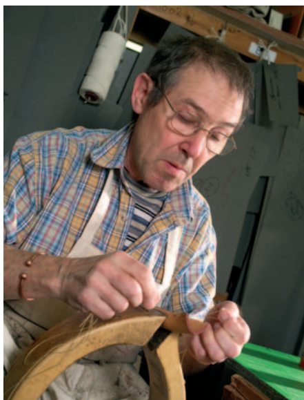
Hand Stitching using Knee clamp
