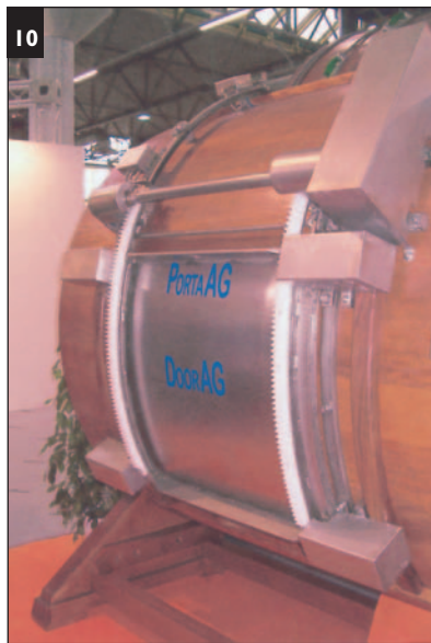
Figure 15 New AG vertical door has no inflatable seals.
