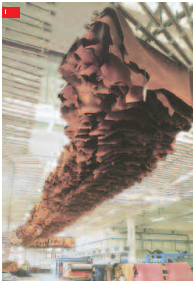
Figure 1: Overhead conveyor systems in a finishing shop (Thema)
