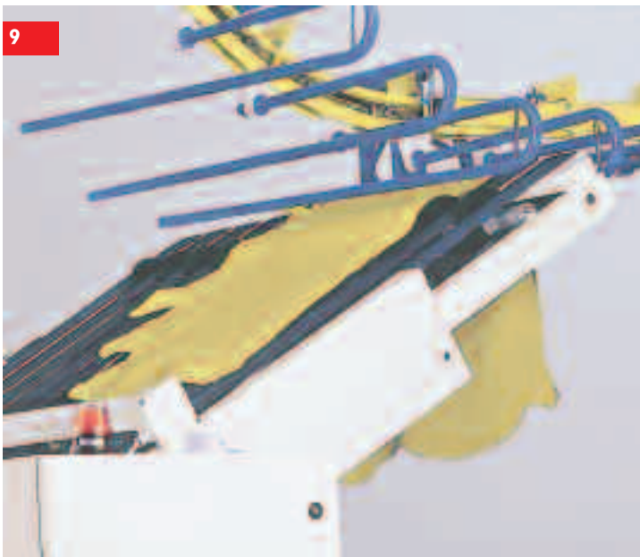
Figure 7: Loading an overhead conveyor from the end of a drying tunnel (Thema)
