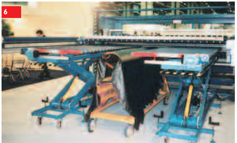
Figure 4: A modern whole hide stacker (Gemata)
