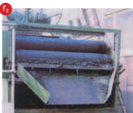
Pressed solids being peeled from the nylon mesh conveying belt of a belt press.
