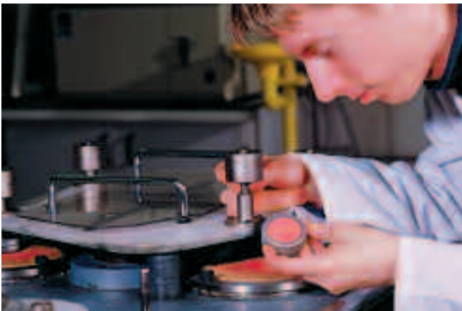
1. The Martindale test, where the outer surface of the mounted leather samples is subjected to abrasive disks under load, being moving in a frame in an engineered configuration.
