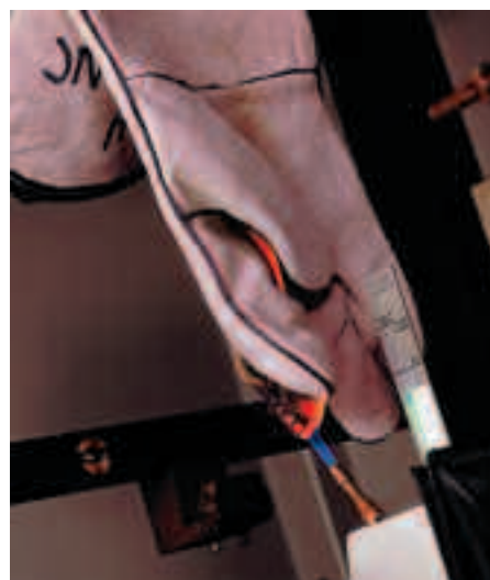
5. The standard flame is applied to the complete glove. Performance is assessed by measuring the time that the glove continues to burn, and the time of after glow.
