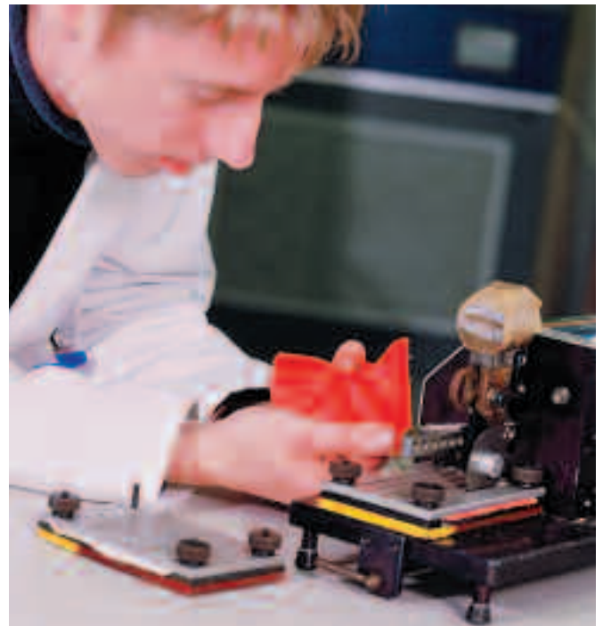
2. The blade cutting test where the performance is assessed by subjecting the samples to a circular blade under load moving backwards and forward across the sample (under inspection) until penetration is achieved.
