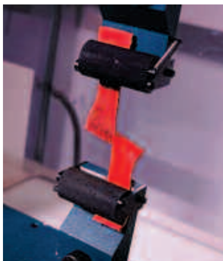
3. Tear resistance, where the load required to tear the leather is measured using the Instron Tensile Strength machine.
