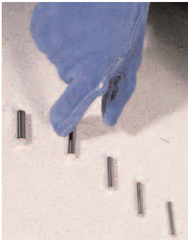
6. Dexterity is evaluated by picking up pins while wearing gloves.
