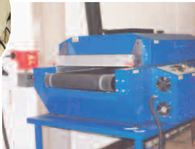
Infra-red and Ultra-violet curing equipment used for development work with powder-based finishing systems.
