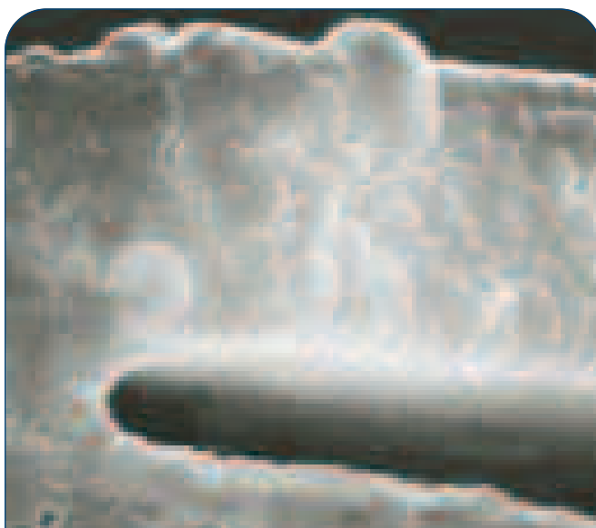
Figure 9: Water based polyurethane resin examined using Cryo-SEM to examine film formation. (Viewed at 9800x magnification).
