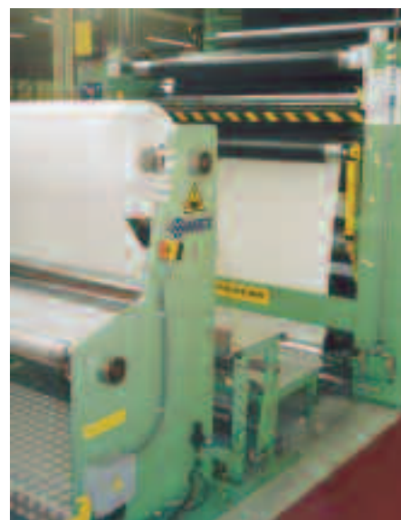
Separation of the foil after finishing from the textured release paper.
