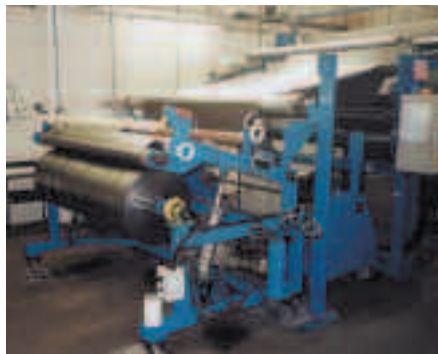
Precise tension is applied to the base-foil as it is wound into a roll.
