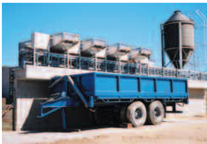
Figure 3: V-Fold filters used to dewater thickened biological sludge at a tannery in Queensland, Australia. The filter cake is composted on site with sawdust.
