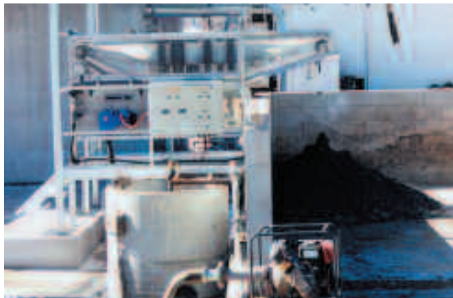
Figure 2: V-Fold filter being used on settled chrome precipitate at a tannery processing 15,000 cattle hides per week to the wet blue state, Queensland, Australia. Typical filter cake production rate is 200 kg/hour at 20% dry solids for disposal.
