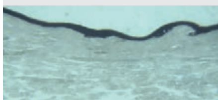
Figure 11: Microscopic examination of a 30 \mu section of non-defective leather. The examination did not reveal the presence of material inside the canals of the hair follicles.
