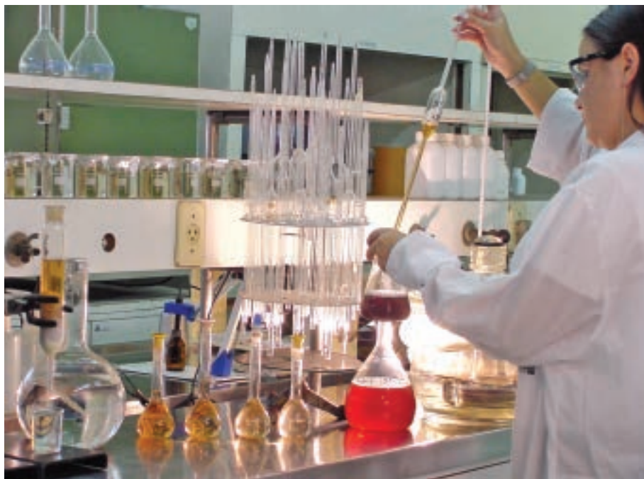
Tannin content analysis being carried out at SETA's Quality Control laboratory.
