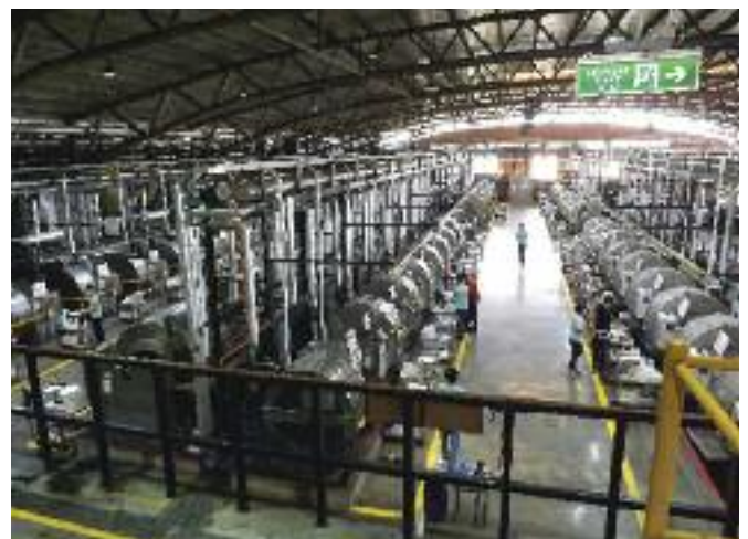
60 trial drums are used to produce the 500,000 square-feet of samples that PAV makes each month. Small orders and order shortfall can also be made up using these drums.
