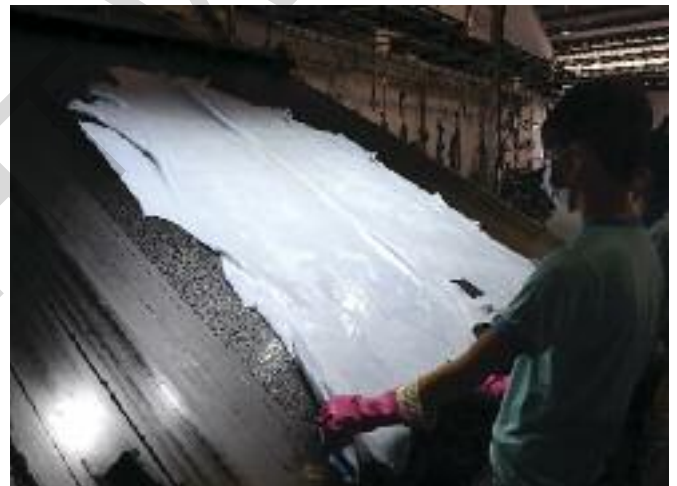
Soaked back, the wet blue hides are inspected on a pitched conveyor. The wet blue is tested for chrome VI every three months with restricted substance and REACH compliance tests twice per year.
