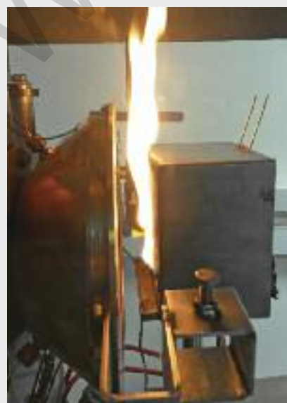
Leather samples and finished products undergoing flame-retardant testing.
