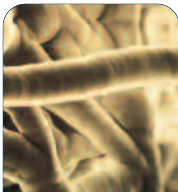
Figure 3: Coated fibrils in a heavily oiled water-resistant leather. (Viewed at 10000x magnification).
