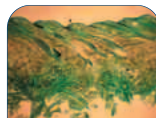
Figure 6: Penetration of syntan into leather structure using Methylene blue.
