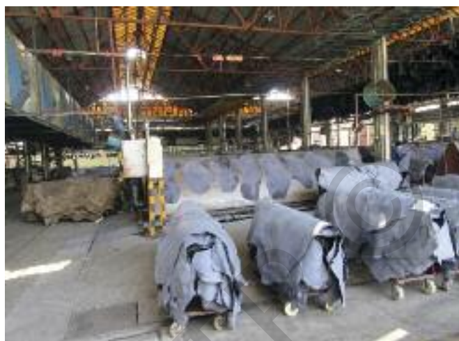
Dyed splits are dried out on heated frames. The open nature of the buildings allows air movement to assist evaporation.
