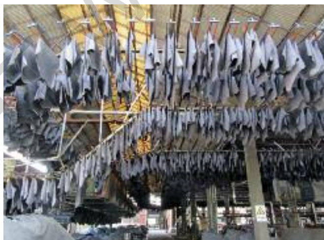
Dyed splits undergoing final drying on one of three 300 metre hanging chain conveyor. The conveyor is used for both drying dyed crust and also airing off pigmented splits.
