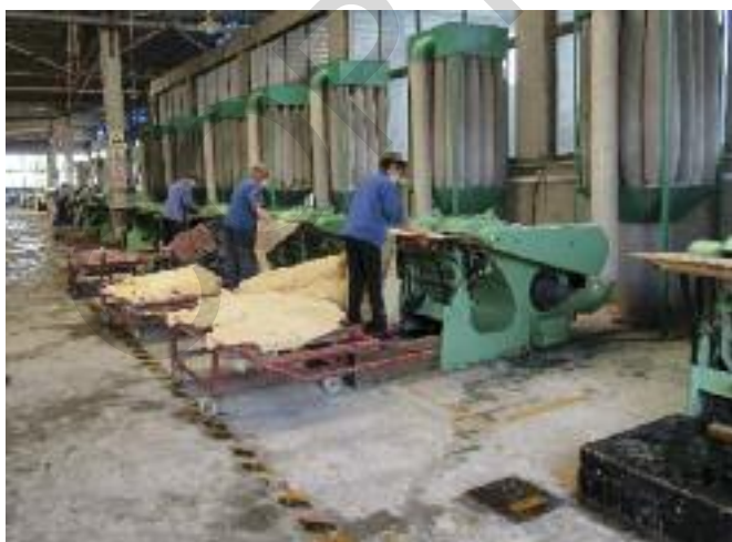
A bank of nine 24" Deep throat buffing machines. The lack of dust is evidence of the efficiency of the extraction units. The area was built in 2014 and underneath it is housed the storage basement for incoming splits.
