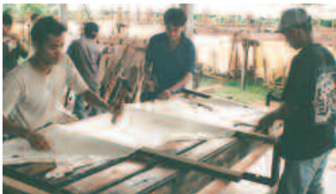
Wet delimed splits being nailed to shape on simple rectangular wooden drying frame set on a table.
