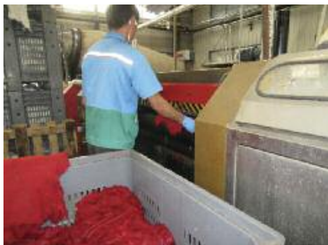
Drained skins are samm set on the flesh side prior to hang drying on the elevated conveyor.
