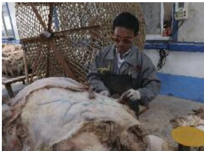
After desalting the skins are trimmed and sorted into piles for further processing. At this stage they are purely sorted into size with any that have ink-based identification marks on the wool put to one side.
