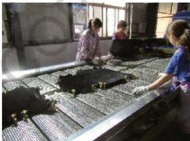
The final stage prior to finishing is an automated toggling that gives a final stretch to the skins. This operation ensures the skins are flat but also allows the area to be maintained.
