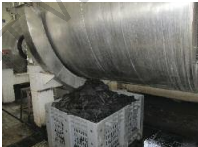
After dyeing, the skins are dropped into slatted Dolav boxes to allow drainage. The boxes are easily lifted by forklift truck and taken to the next stage of the processing. It is in similar boxes that the chrome tanned skins are also held prior to further mechanical dewatering.
