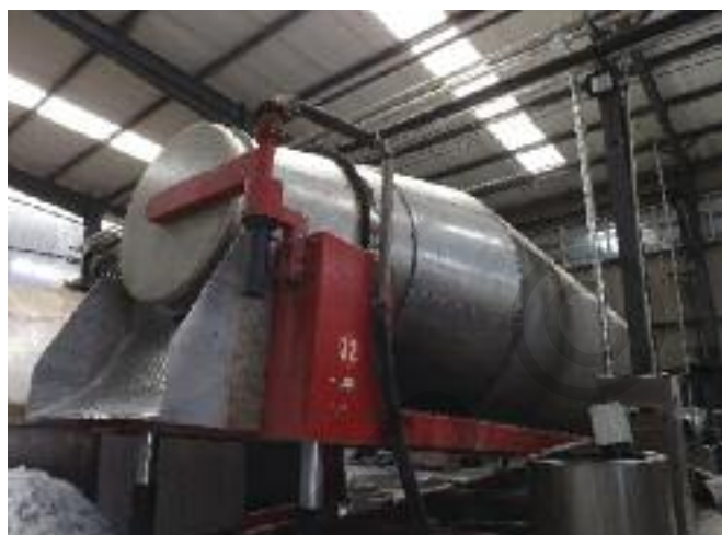
Reputed to be the largest in China, this hide processor can tan up to 3,000 skins at a time. Whilst rotating in one direction, the gentle mechanical action aids the tanning without felting the wool. When run in the opposite direction the Archimedes screw type arrangement of the blade discharges the contents.
