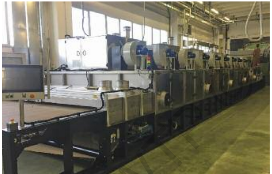
The RF dryer works at a maximum belt speed of 12 metres per minute, drying hides in minutes rather than hours. CREDIT: CARTIGLIANO
