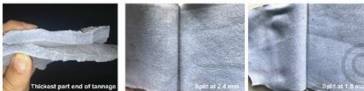
Fig 15: Picture of thickest part of the wet blue and splits at 2.4 millimetres or 1.5 millimetres.
