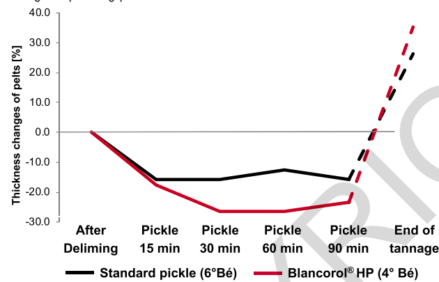
Fig 11: Thickness change of the skin as a measure for the swelling during the pickling process.
