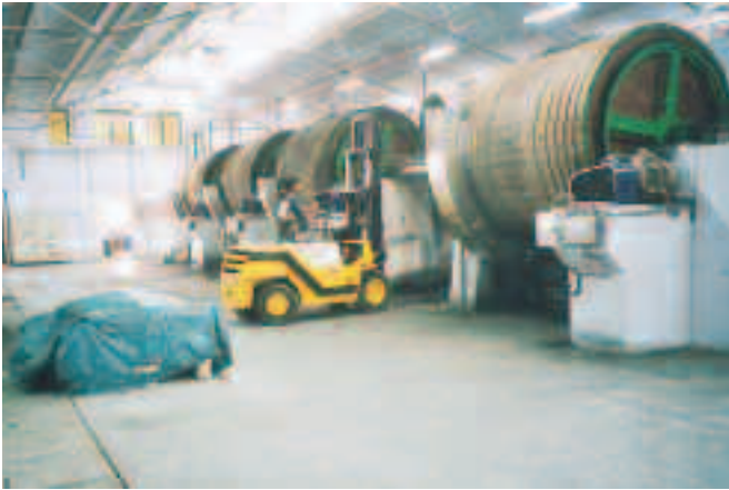
The movement of all leather between drum processing and machine operations is by forklift truck using specially designed and reinforced pallets. A mezzanine provides servicing for the processing drums.
