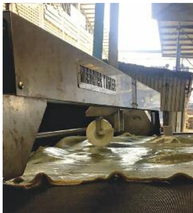
Continuous analysis of the hides allows the machine to autocorrect for any changes in the limed pelt prior to splitting.
