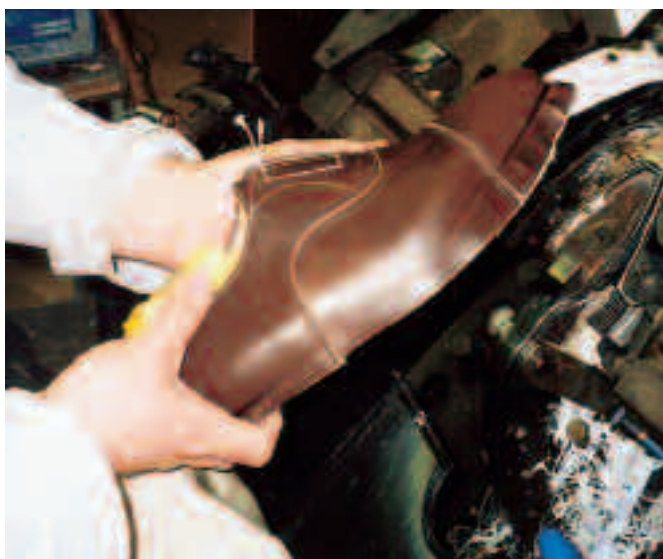
Figure 5 By exploiting the elasticity-plasticity balance of leather, a flat component can acquire a new three dimensional configuration. This photo shows how a leather upper is pulled and moulded over the last on a men's Goodyear welted shoe.
