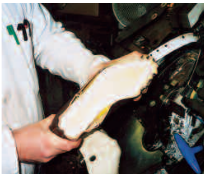
Figure 6 This underneath view shows the upper bonded to the insole rib. The upper is further attached to the rib at seat and waist prior to welt sewing. The leather then uses its set properties to maintain the new three dimensional form.
