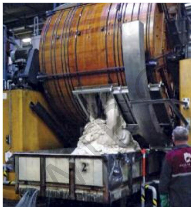
Unloading hides from one of the Hüni drums. Production of chrome-free leathers is also part of the operation.
