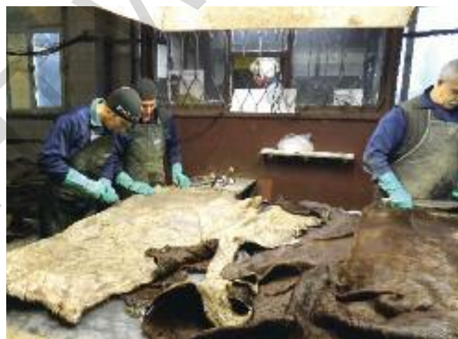
Hide inspection and grading identification on purpose-built lighting stages. It was noticeable that the hides were quite small but looked clean of dung suggesting good animal husbandry. The grade stamp is noted in the adjoining small office and entered on the computer system.
