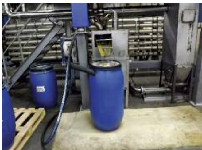
25 tonnes of limed fleshings are treated every day and from this approximately 90 tonnes per month of industrial fat is produced and sold for use in soaps, cosmetics and animal feeds. The resultant waste cake is used for fertiliser whilst the water goes back through the effluent treatment plant. This is also an excellent reuse of barrels that contained the processing chemicals.
