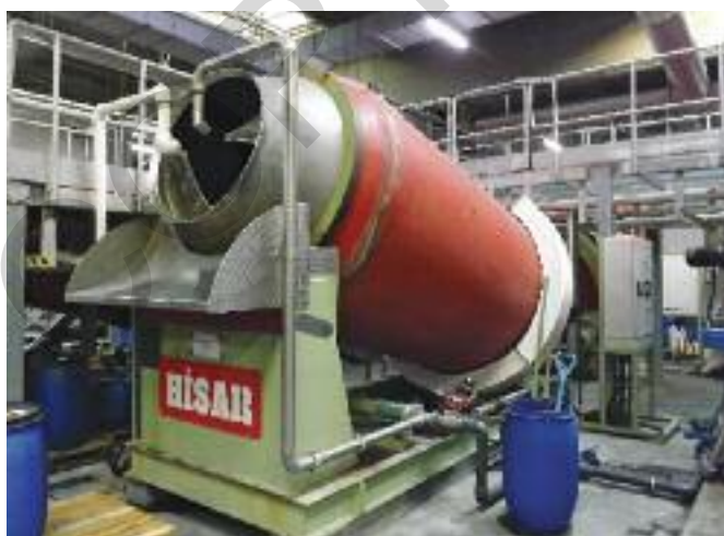
The processing of sheepskins, approximately 5,000 per week, in a newly constructed area within the tannery. Although separate to where the hides are processed, the waste waters are treated together with the soak liquors being reused after primary treatment.
