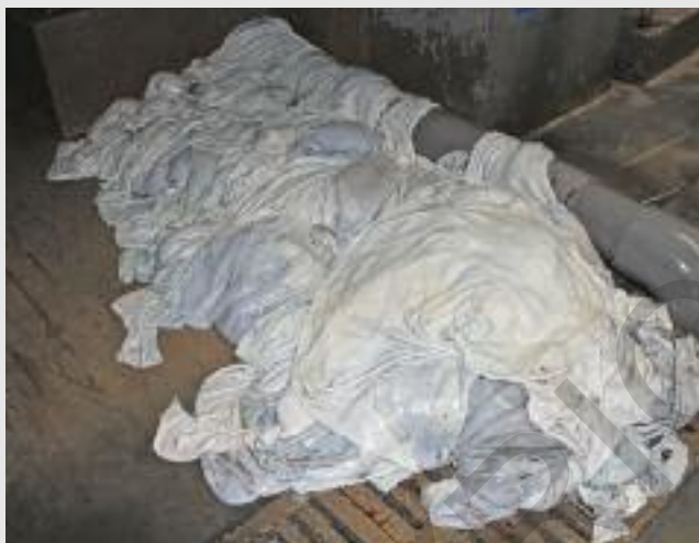
Delimed hides: salts, residual proteins and fats are released from throughout the structure during the deliming and bating process.
