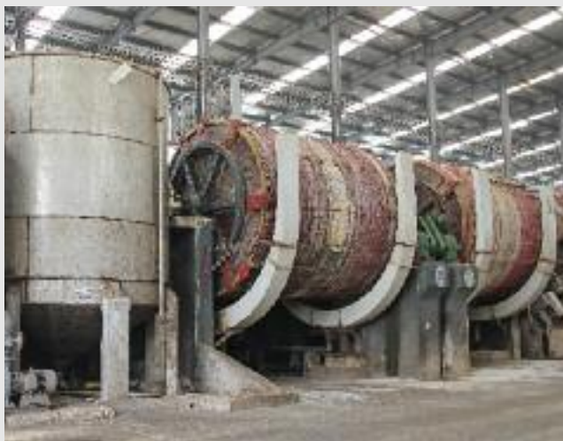
Collection tank used for recovered floats from all of the liming drums on completion of the hair recovery liming process.
