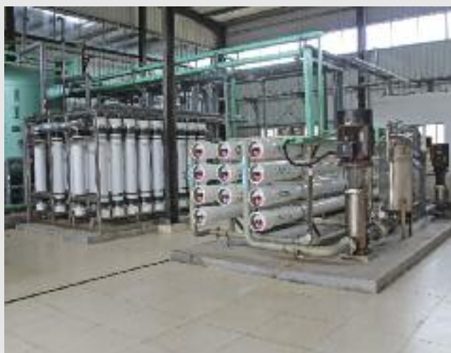
The reduced volume and salinity at the end of primary and secondary effluent treatment significantly reduces the load on membrane filtration and reverse osmosis when used as tertiary effluent treatment.
