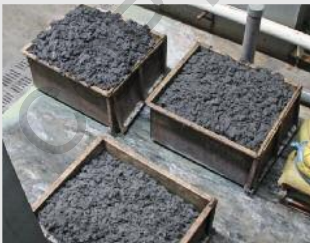
Compact dewatered and uncontaminated hair following hair recovery. This operation significantly reduces the volume of contaminated sludge for disposal at the end of effluent treatment.
