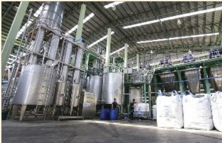
Technology that IHL has set up converts chrome shavings into recycled chrome and also generates a new filler product that Interhides is using in tanning, retanning and finishing.
