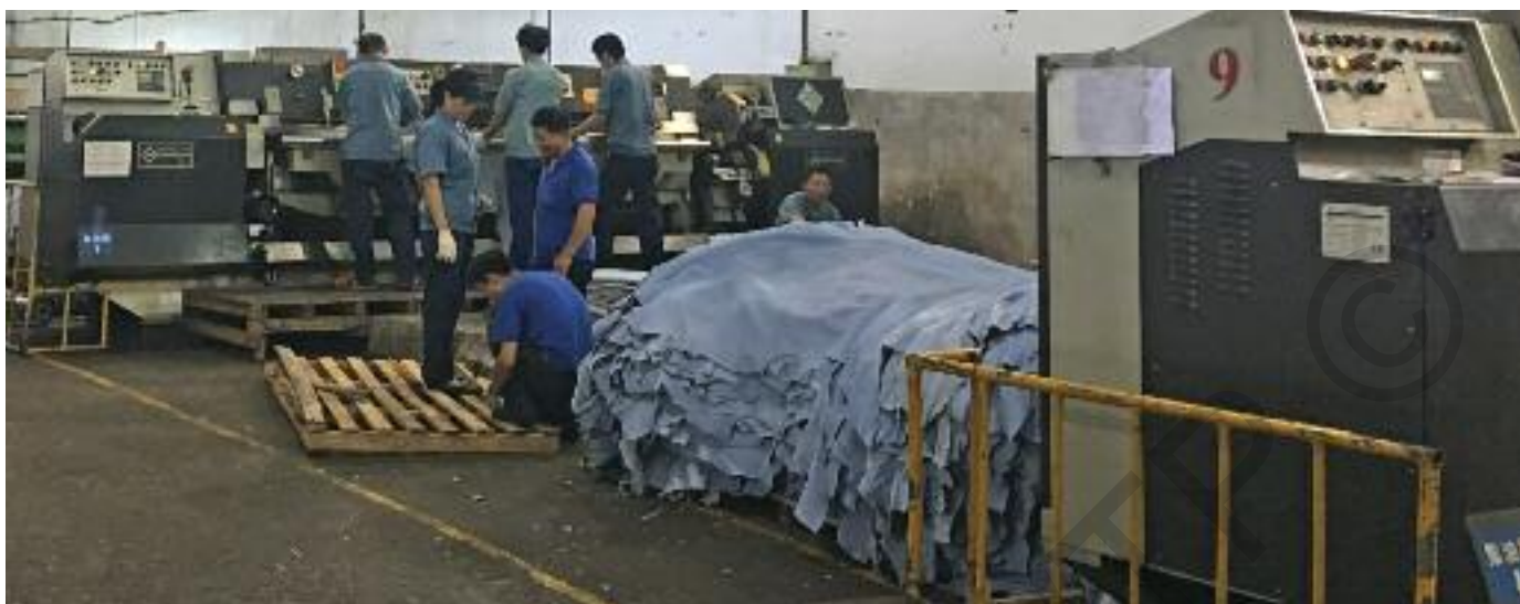
Wet blue splitting at a tannery in China. CREDIT: XINGYE
