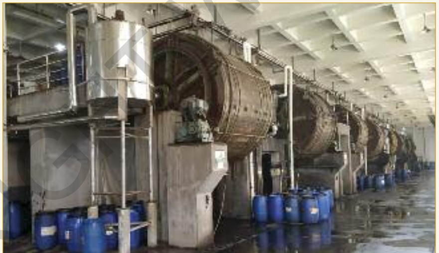
Retanning drums with some level of automated control at the Andong tannery.
