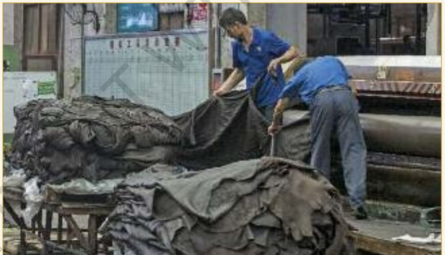
Locally made tanning machinery is also in use at TTX, in the wet stretching operation, for example.
