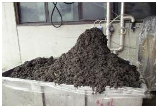
Figure 2: Hair recovered from unhairing process.
