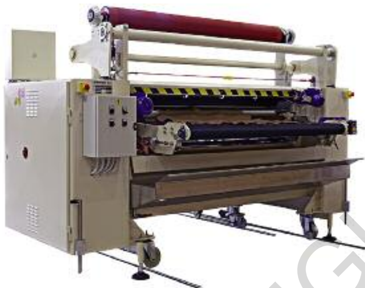
Rear view of the Deepcolor showing the two cylinder arrangement.
