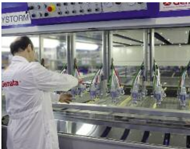
Accessible array of spray guns and arms holding guns.
