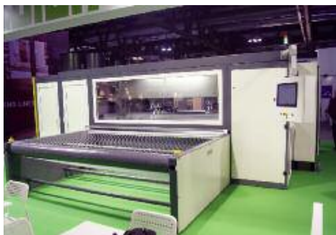
Front view of spray cabin. Spray mechanism with see-through window.
