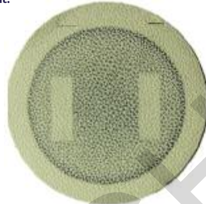
Panel 1: Rub tracks after effected cleaning. Leather Sample 2 (beige) with coarse embossment.
