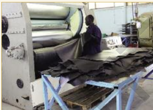
After roller coating, and spray coats, leathers are finally embossed using a ram press, or lightly rolled as shown before final inspection, area measurement and delivery to the footwear plant.
