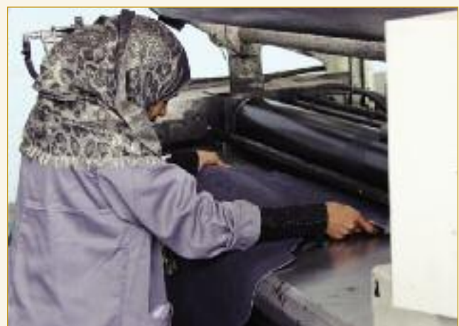
The finishing department is equipped with a new roller coating machine for applying base coats, followed by a steam drying cabinet. In addition there are two new spraying lines with drying tunnels fitted with a cooling zone.
