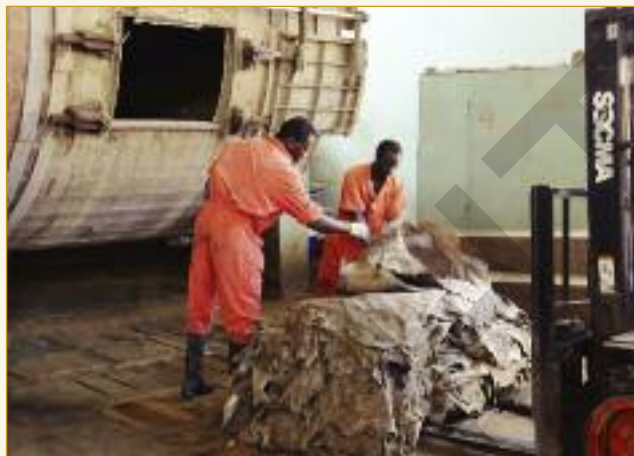
Drums are used for soaking and unhairing/liming bovine hides in a 48-hour cycle. Air dried and dry salted hides are pre-soaked in pits served by overhead hoist before transfer for drum processing.
