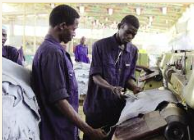
All sides are sided after samming and grading, and then shaved by a team of two operatives to minimise damage to the flank parts. Every fifth side is checked for substance.
