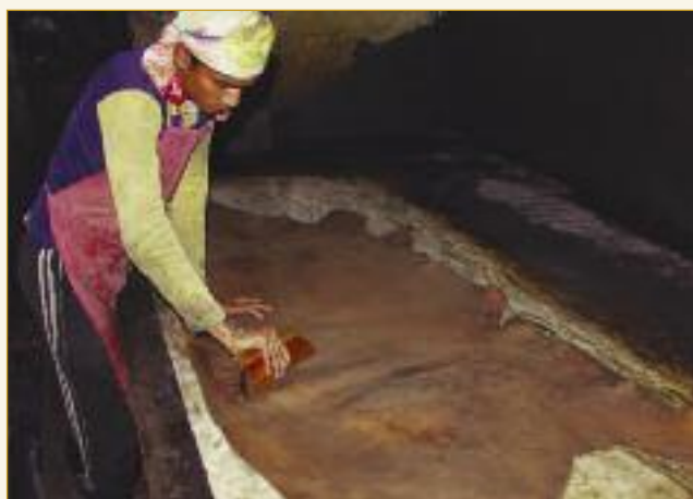
The dried vegetable tanned saddle leathers are lightly rewetted, then set out by hand in preparation for a hand oiling of the grain with linseed oil.
