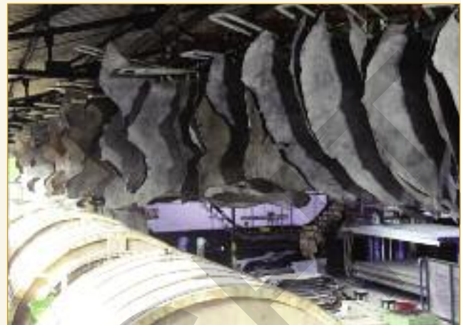
All of the leathers are dried naturally in the roof areas of the tannery. The movement of the conveyor system is operated by a 1-HP electric motor.
