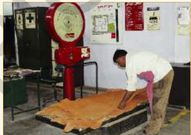
On entering the finishing department all leathers are measured for area, then weighed as part of process control.
