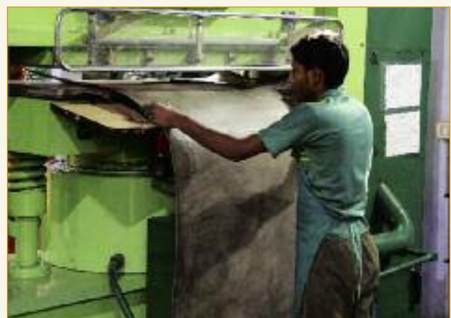
Many of the leathers produced are ram pressed both to consolidate the structure and to develop the gloss.
