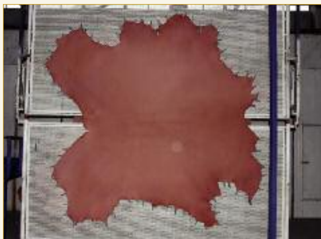
All of the automotive hides are toggle dried, and sold in the pre-finished state.
