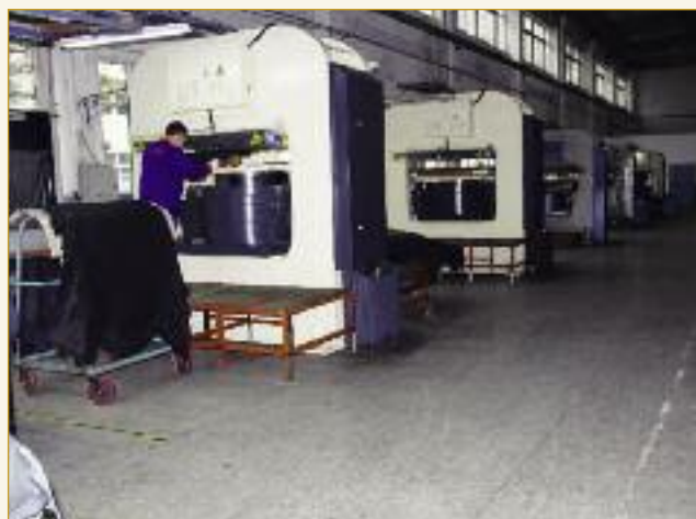
In addition to four roller presses, five embossing machines are used within the upper leather finishing plant.
