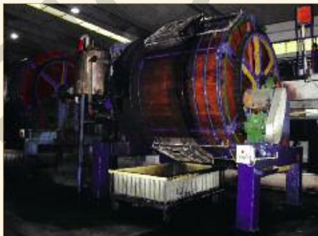
Within the dyeing department there are two new tri-section wooden drums, fitted with stainless steel Y-section interior divisions. Each vessel has a capacity of 200 hides per load.
