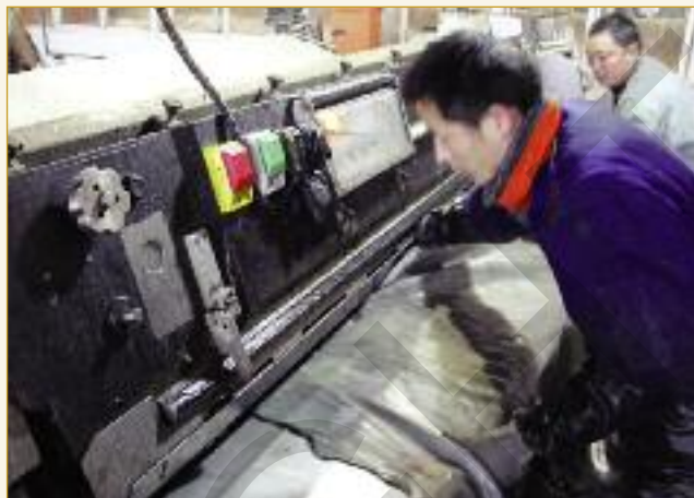
All of the hides are fleshed after soaking, and then split after a hair-burn liming.
