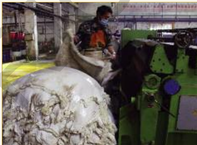
After soaking and draining, all of the sheep skins are first time fleshed which also flattens and extends the skins. They are then wool sheared to length, then fleshed a second time as shown to create a very clean and uniform flesh part.
