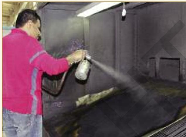
Some hand spraying operations are performed, but these are mainly for development work.
