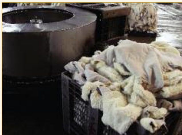
After retannage, centrifuges are used to dewater. This operation is followed by a light samm/set to stretch and remove all creases before wheel-buffing.
