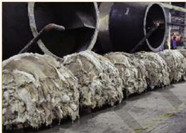
Wet salted sheep skins are soaked in a batch of steel woolskin processing drums. Dry salted skins are less flexible at this stage and need soaking in paddles.
