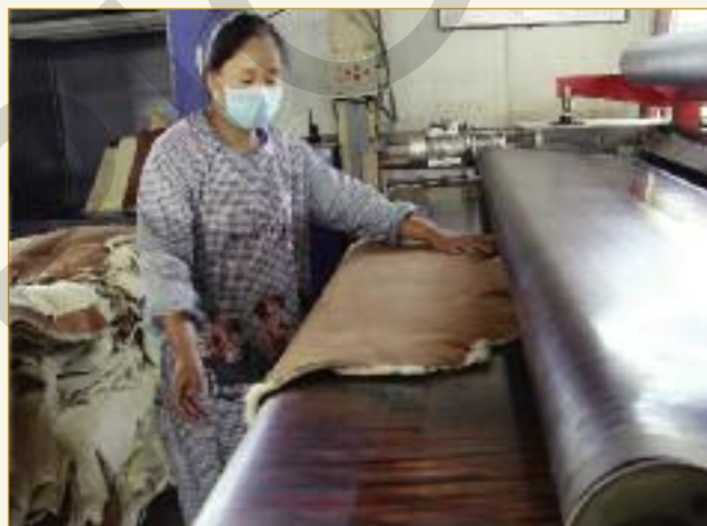
The suede side is treated with fixatives in finishing to improve colour fastness. Both spray application and roller coaters fitted with a belt feed arrangement as shown are used.
