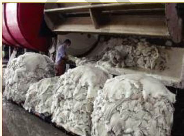
All of the retanning and fatliquoring operations are performed without any dyestuff additions. These tipping paddles are designed to enable a fast unloading of these natural skins with minimum handling strain for the operatives.
