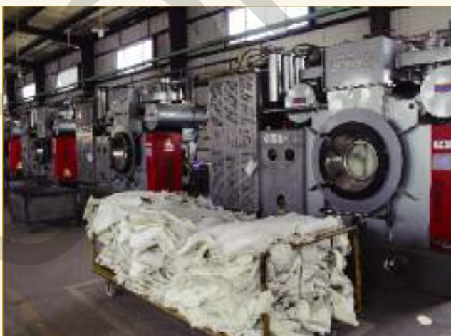
After first time drying, all of the sheepskins are solvent degreased in a three hour operation; 11 degreasing machines are used at the moment, and this stage is followed by wool and leather dyeing.
