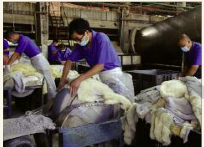
All of the sheepskins are wheel-buffed to remove fibre and extend the skin structure. This takes place after chrome-free tanning, retannage/fatliquoring (as shown) and in the dried state in conjunction with wool carding/shearing and ironing operations.
