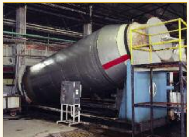
These dyeing machines are suitable for both dyeing the wool and dyeing the leather. The number of sheep skins in each load is between 600–900, and can be compared to 200 in traditional paddles used for dyeing.
