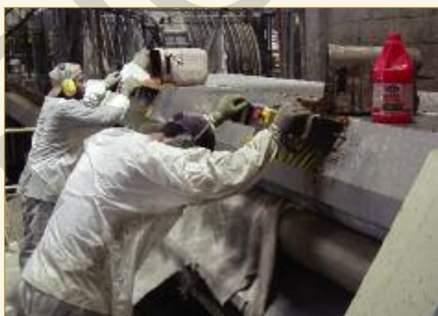
Within the fleshing operations, as part of operative safety, both operatives need to place and retain both of their hands on pressure pads set on machine (as shown) during the machine closure phase.
