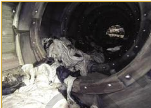
Salted hides together with water are moved through this wetting back drum on rotation to rehydrate the hides in preparation for the green fleshing operation.
