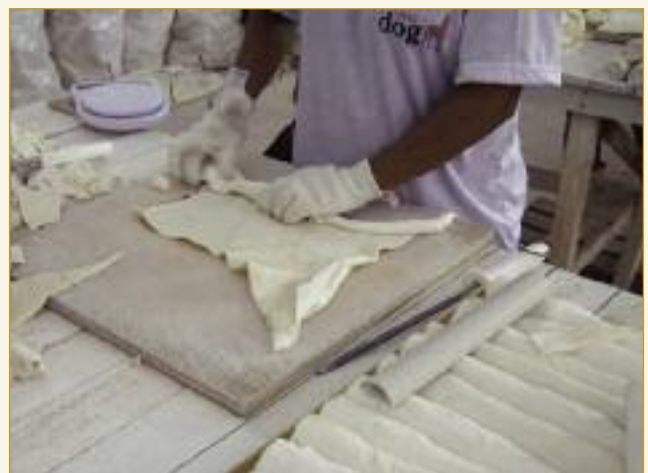
Dog chew products are manufactured on site. Photograph shows limed splits that have been bleached and delimed, are then cut to size and hand-rolled before drying.
