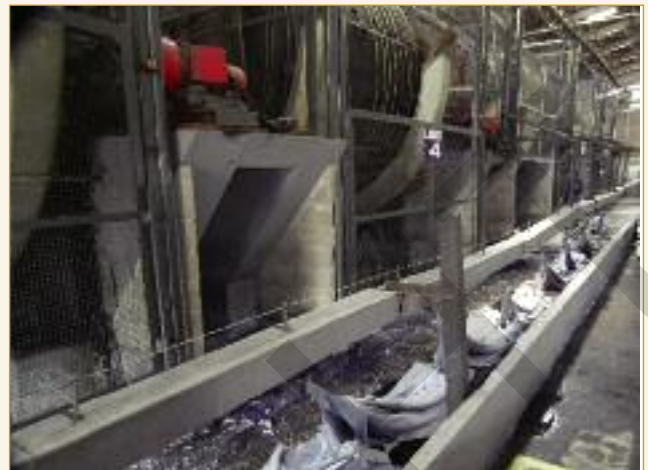
After dumping the hides beneath the tanning drums after chrome tanning, they are hooked onto a line-conveyor for direct feed to the samming operation.
