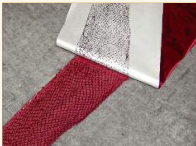
The fish skin production is very dependent upon accurate dyeings, but many other finishing effects are created including the use of foil laminates.
