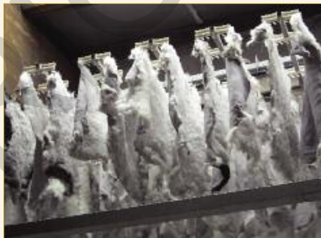
Both the shearlings and wool skins for rugs are dried tension-free on the overhead conveyor system.
