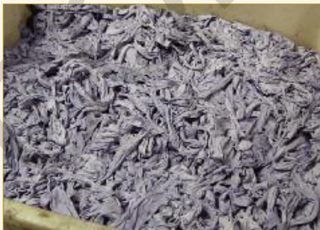
All of the fish skin leathers are chrome-tanned, with the residual chrome-containing wastewaters segregated and precipitated within the tannery building.
