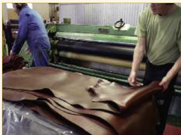
After drum stuffing, all of the hides are set two ways on the flesh side, then two ways on the grain side to flatten and enhance the final grain appearance.
