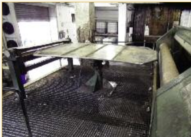
All lime fleshing is performed on a single conventional out-feed Rizzi fleshing machine. The handling arrangement is unusual as hides are slid into the machine from a feed table. On out-feed, the hides are guided back onto this table, which is then rotated 180 degrees. The neck end is then fed into the machine to complete the action.
