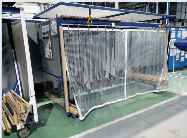
Here, leather placed on poles during finishing and held in this mobile frame is enclosed using hard plastic and curtaining materials to avoid dust associated problems.
