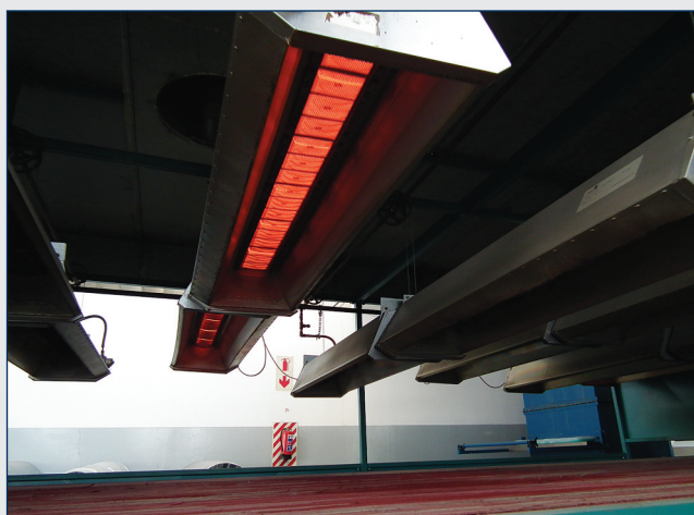
Infra-red drying is a fast evolving technology, minimising air movement over wet finish films and hence the risk of dust adhering to the wet finish film.
