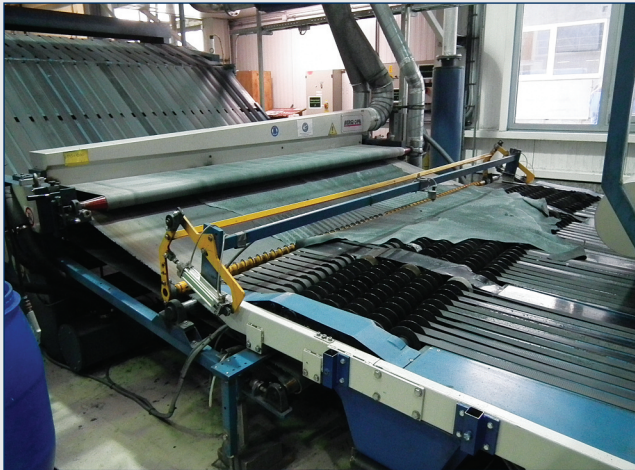
Efficient dust extraction, collection and earthing of equipment is essential within de-dusting operations after buffing.
