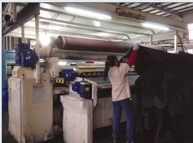
Feed-area for finish applications are being fitted with overhead cover, and the ability to fit side cover and curtains to enable complete isolation.
