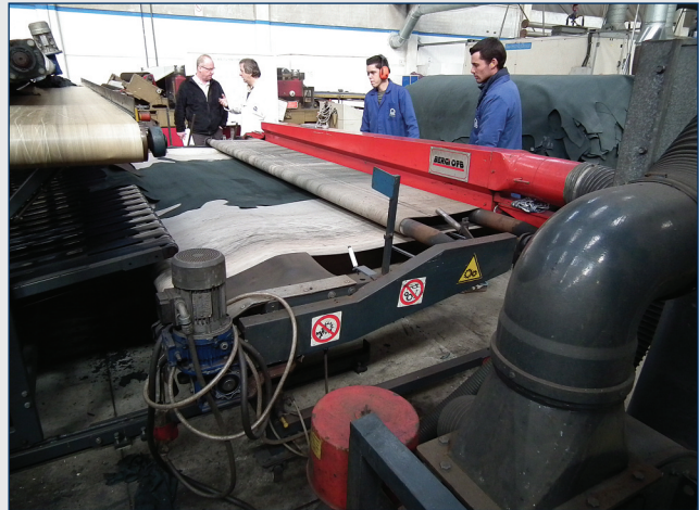
Dust removal is being employed as part of dry splitting operations where very accurate leather substances are essential.
