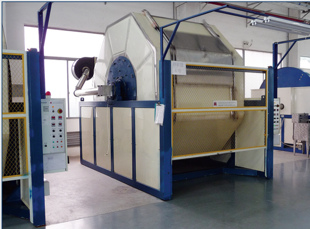
Milling operations are also a source of dust and fibres. In this example the dust collection is external, although the filtered air at controlled temperature and humidity is returned back into the drum.
