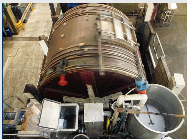
Image shows dust and fibres being filter screened from the float during recirculation within the retanning process.
