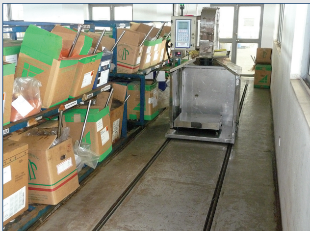
Scales fitted with dust extraction that can be readily moved on rail track to the appropriate dye container is an effective innovation to avoid dust. This is also being applied to weighing areas for other dry chemicals.
