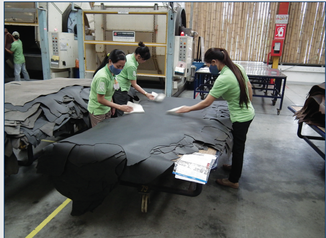
Even in the best conditions, sometimes dust needs removing at some point, in this case by hand using tacky cloths.
