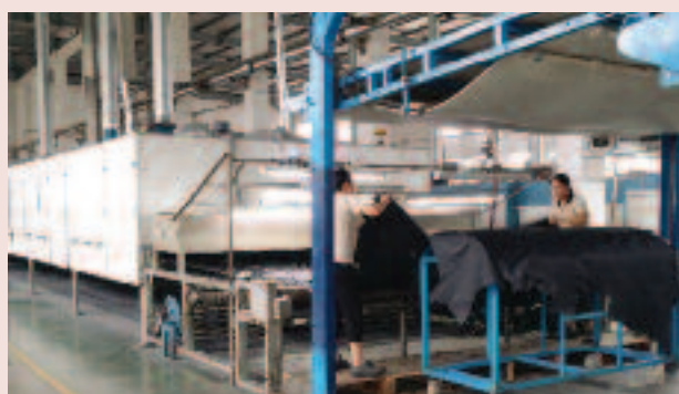
There are three Mega Star Gemata roller coating machines used in the finishing department at Chinese tannery Zhejiang Mingxin . The roller coating drying cabinets are set in tandem with spraying lines. These can be linked together by lowering the overhead bridge arrangement.
