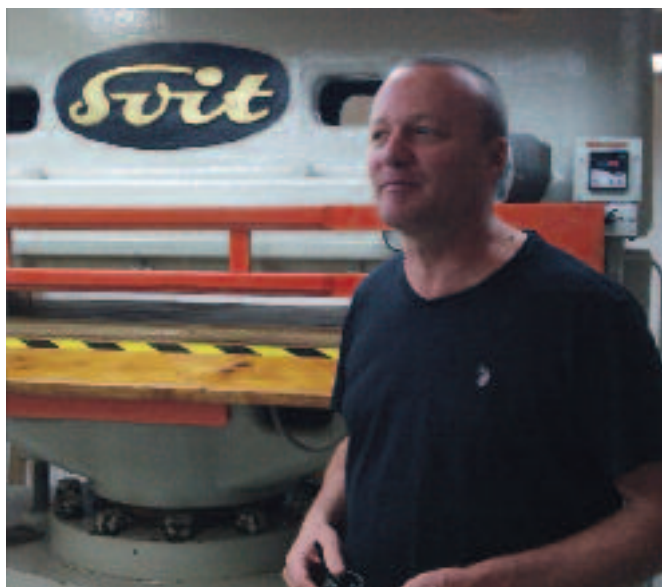
Leandro Scur believes older machines, like this 60-year-old Svit embossing machine that he restored himself, are well suited to tanning exotic skins.
