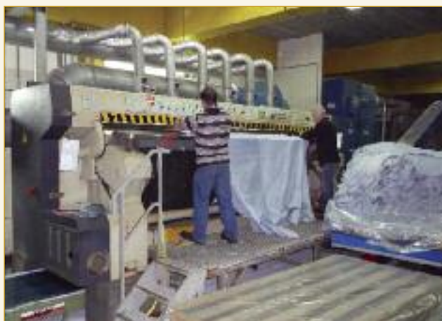
Blue shaving of hides with dust control for in-house manufacture.
