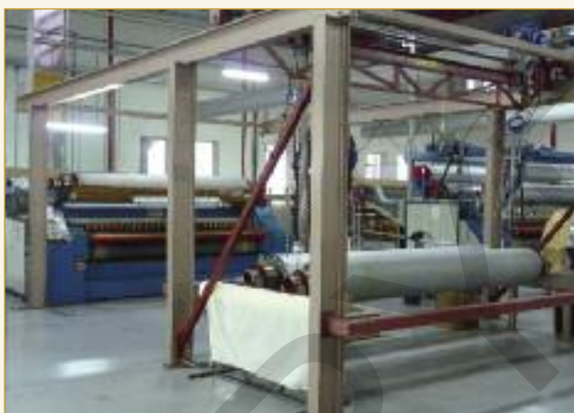
It takes five minutes to change the embossing rollers using this hoist and gantry arrangement. This technique has been built into the design of the Bergi Supra Press in the Hulshof finishing department, where five rollers are built into the machine.
