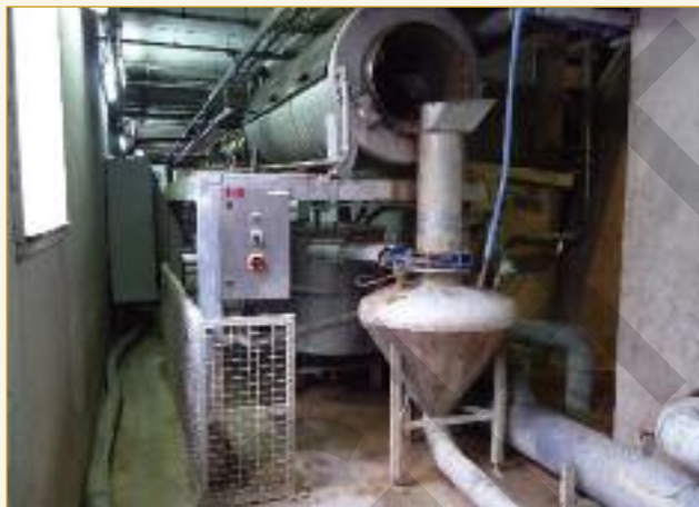
Hair is recovered using a rotating screen. To avoid the risks of contamination in an area operating to the standards required for food production, the recovered hair drops into a cyclone to be blown away from the processing area.
