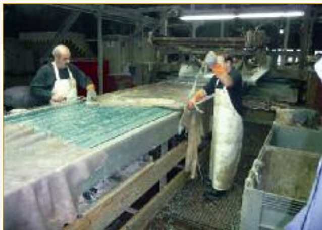
After fleshing, the hides are limed trimmed on a conveyor as they are delivered to the lime splitting operatives.
