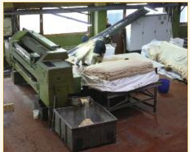
Shaving wet white leathers. The shaving are collected and used for "free-of-chrome" leather board.
