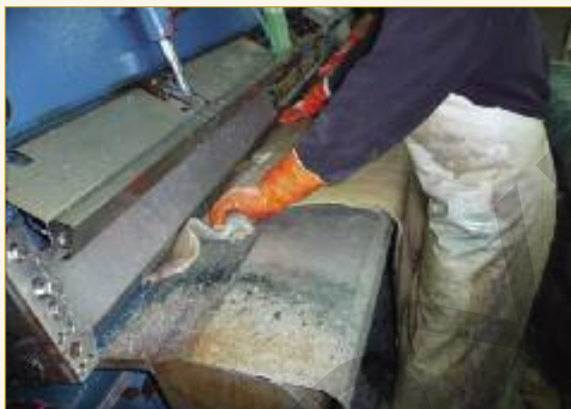
After lime splitting, the grain splits are conveyed from the area for tanning, and the flesh splits conveyed to the split trimming area.
