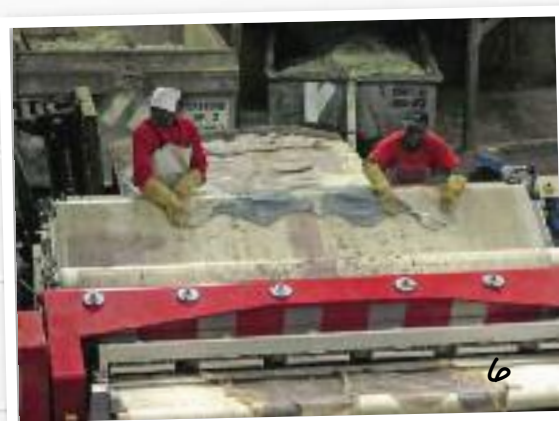
5 + 6) Views of operators feeding the splitter using the raised feeding device.
